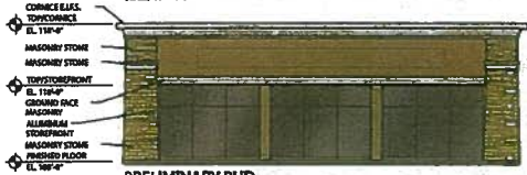
PRELIMINARY PUD BUILDING 'C3' EAST ELEVATION SCALE 1/8" = 1'-0"
