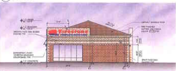
16 RIGHT SIDE (EAST) ELEVATION SCALE: 1/8" = 1'-0"
