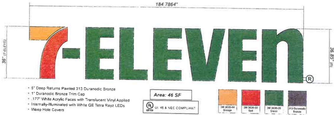
Front View & Side Mounting Detail -CL36REM 36" Internally-Illuminated Remote Channel Letters - Sign C 1/2" = 1' 0" *Must be printed at actual size for scale to apply
