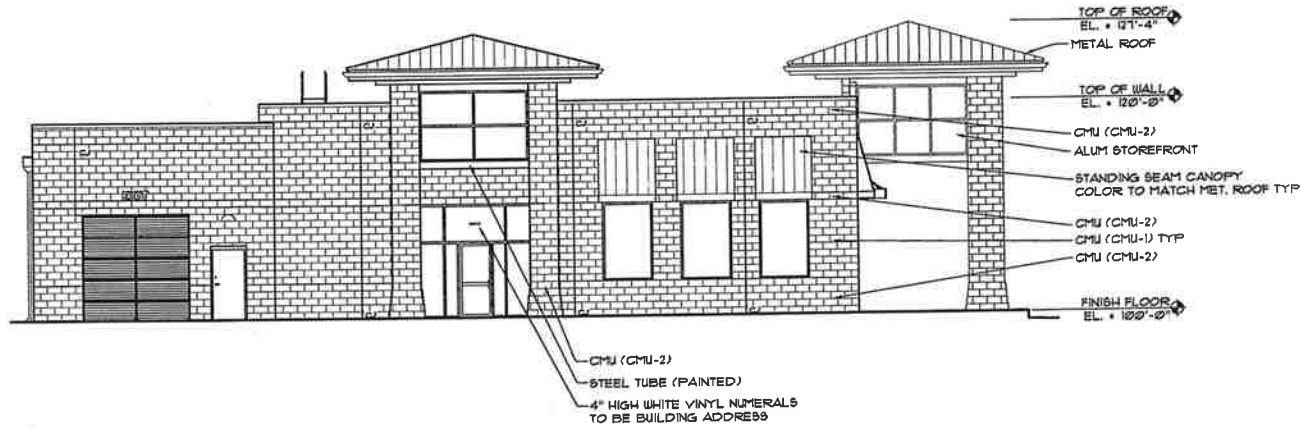
LEFT BUILDING ELEVATION (EAST) SCALE: 1/8" = 1'-0"
