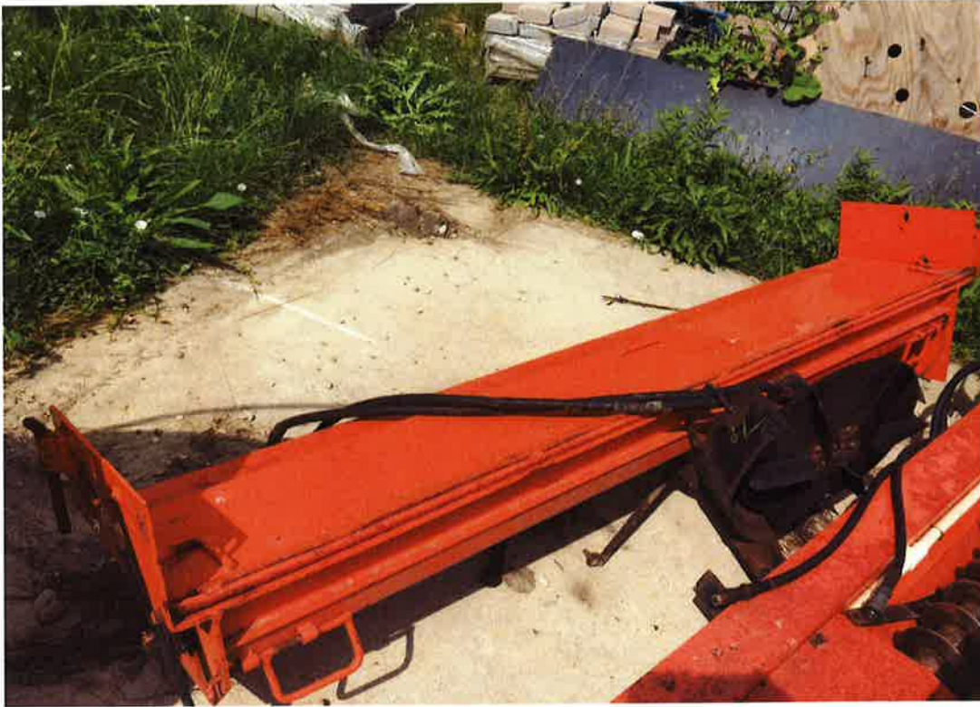
2003 Monroe tailgate spreader with 6" reverse flighting auger.
