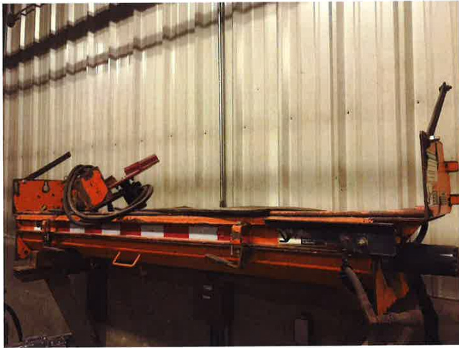
2003 Monroe tailgate spreader with 6" reverse flighting auger.
