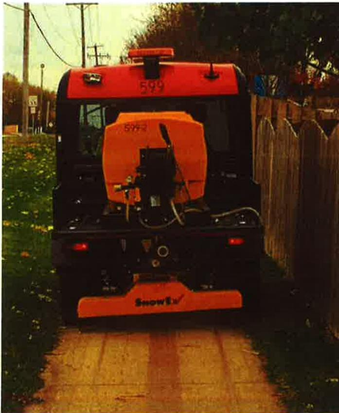
**Four anti-icing units can be deployed – three on roadways and the newest unit for sidewalks and Village properties (pictured here)**
