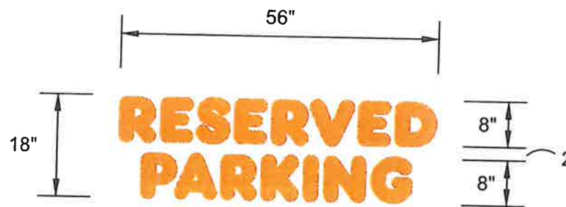
"RESERVED PARKING" SHOULD BE PAINTED ON THE TOP OF THE PARKING STALL (CURB SIDE) SCALE : N.T.S.
