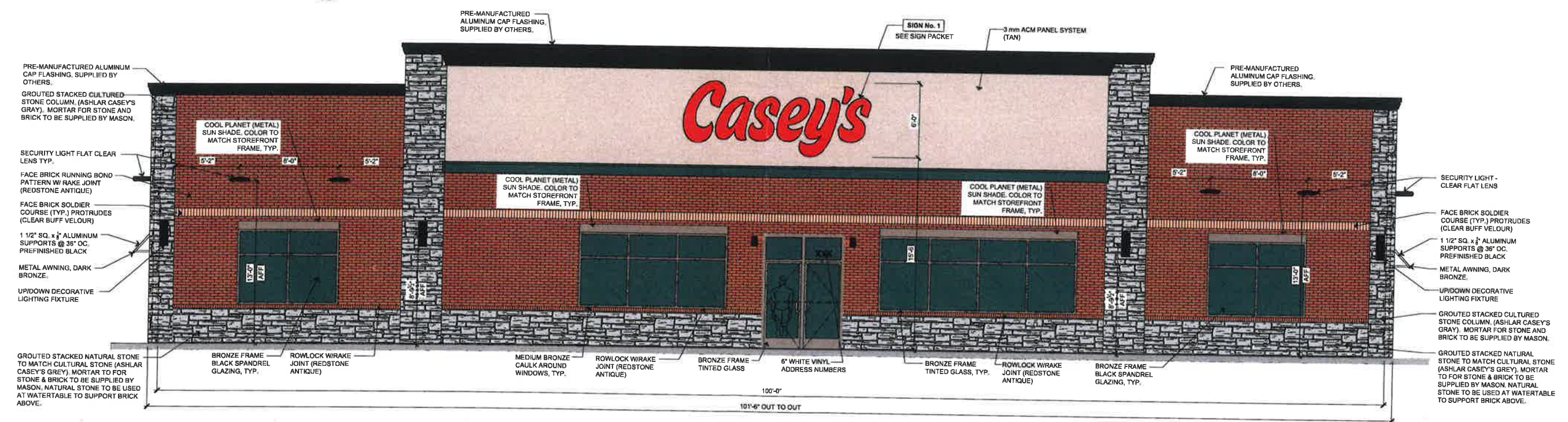
1 Exterior Elevation - Front of Building (Plan West) 1/4"=1'-0"
