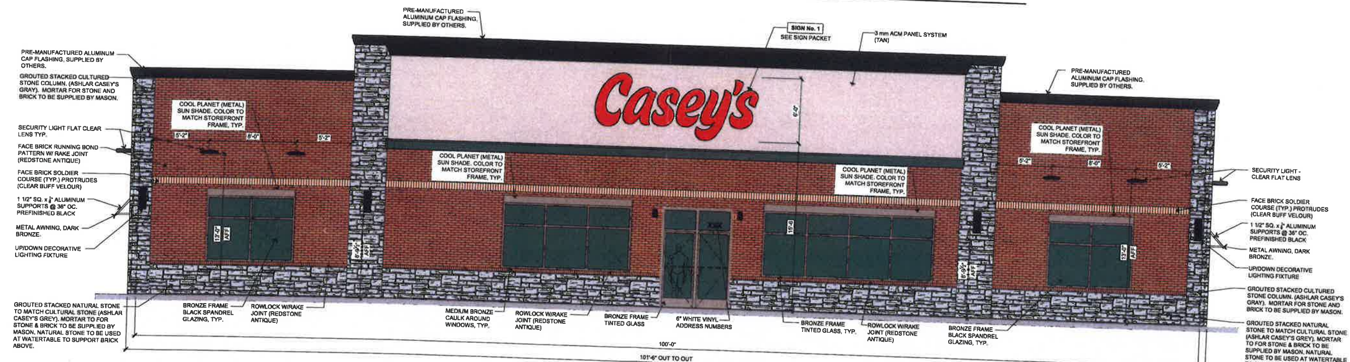
1 Exterior Elevation - Front of Building (Plan West) 1/4"=1'-0"
