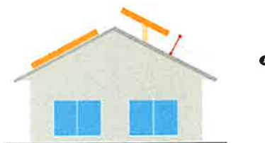
Building-Mounted Solar Energy System 16-5-9(A)
