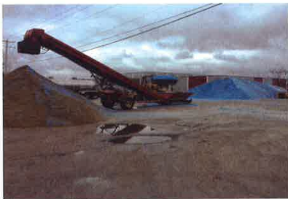
Salt treated with organics before loading in the salt dome
