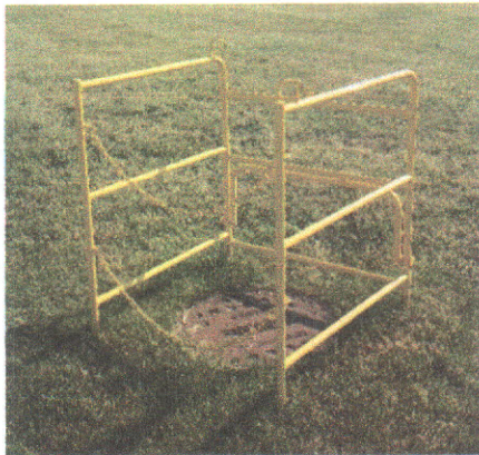
Safety manhole protection.
